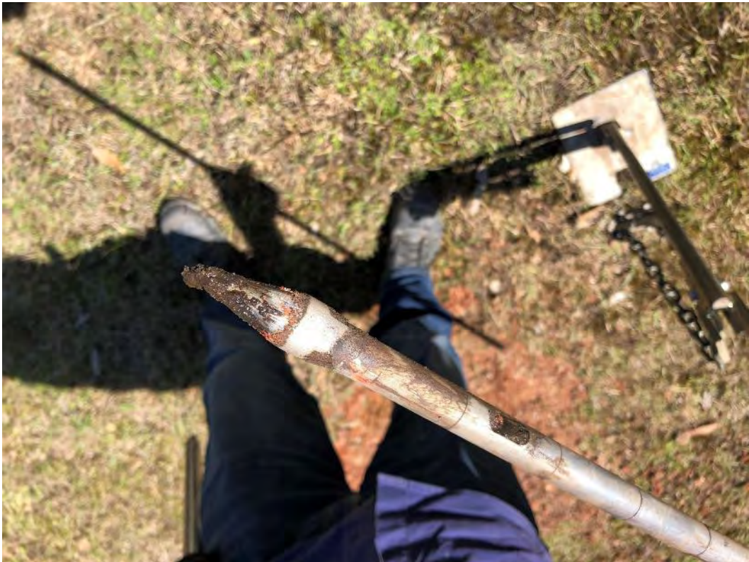
Photograph 8: Natural material encountered on DCP tip.
